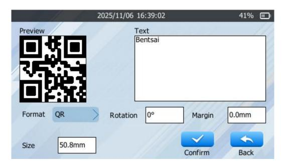
Tap **Add** then select **2D Code**. Enter the string in the text field to generate the code. Below the preview panel, choose the encoding format and configure relevant parameters. Once finished, tap **Confirm** to place the generated QR code onto the canvas.
