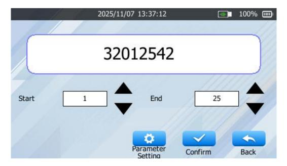
**Start Row Number**: The default value is 1 and can be adjusted by Taping, in increments of 1.
