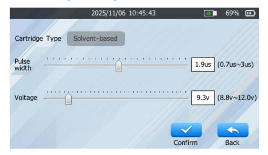
The device automatically detects whether the cartridge is water-based or solvent and applies the corresponding settings. Manual adjustment is typically unnecessary.
